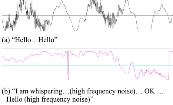
Figure 7. Two real examples of LDV acoustic signals with both low and high frequency noises.
