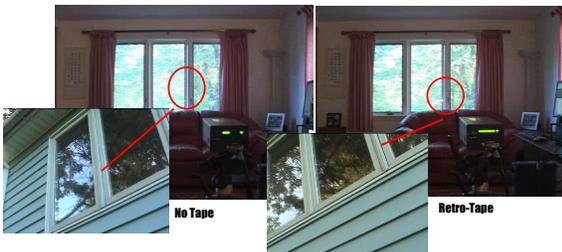
Figure 12. Listening through windows – a person was speaking outside the house, close to a window, while the LDV was listening inside the room via the window frame. Left: without retro-tape; right: with retro-tape.
