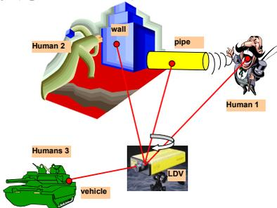
Figure 6. Target selection and multimodal display. The LDV can measure audio signals from tiny vibrations of the LDV points (indicated by the read beams and dots onto the objects) that couple with the audio sources
