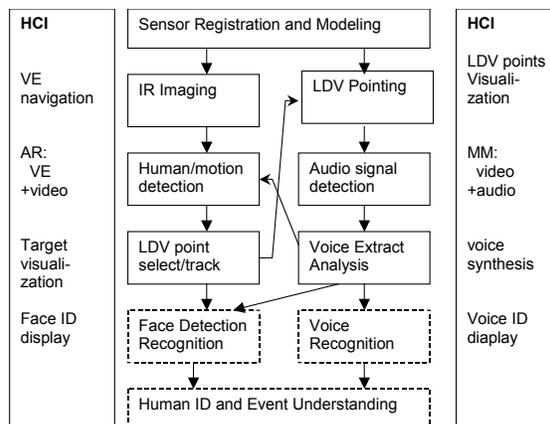
Figure 1. System components of a multimodal human signature detection system.
