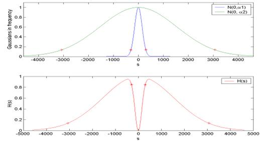
Figure 8. The Gaussian bandpass filter transfer function
