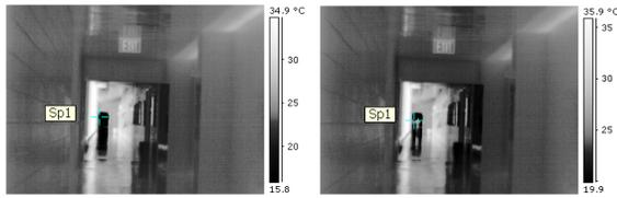
Figure 4. Two IR images before and after a person standing at a distance of about 200 feet. The reading of the temperature at the cross (Sp1) changes from 11°C to 27°C.
