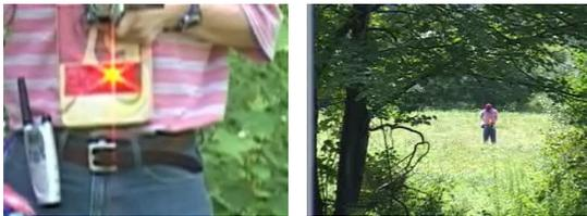
Figure 11. Long range LDV listening experiment. A metal cake box (left) is used, with a piece of 3M traffic retro-tape pasted. The laser spot can be clearly seen.
