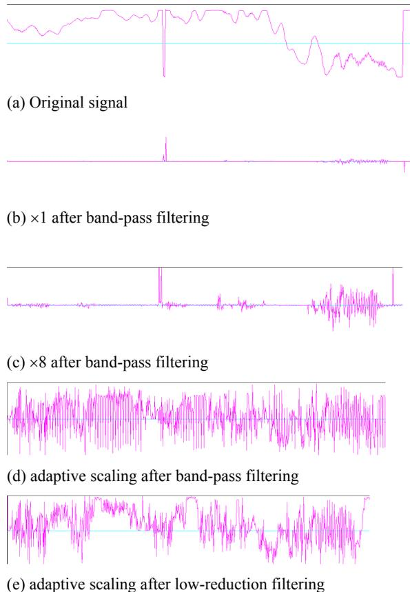
Figure 10. The waveform of the original signal and the results of fixed scaling and adaptive scaling, after using suitable Gaussian filtering. The short audio clip reads “I am whispering... (noise)... OK ... Hello (noise)”, which was captured by the LDV OFV-505 from a metal cake-box carried by a person at a distance of about 30 meters from the LDV.
