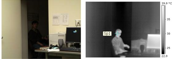
Figure 3. A person sitting in darkness can be clearly seen in the IR image, and the temperature be accurately measured. The reading at the cross (Sp1) on the face is 33.1°C.
