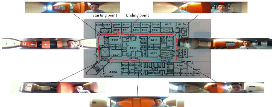
Fig. 1: One testing environment and some sample omnidirectional images. The red line in the map is the modeled path, and the dark blue line as well as the light blue line are the testing paths
