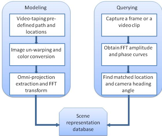
Fig. 4: Work flow of modeling and querying stages
