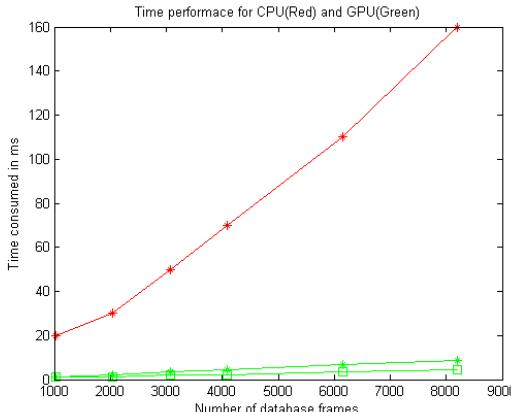
Fig. 8: Time usage with and without GPU acceleration: Red without GPU; Green with GPUs. Curves with squares are experiments using 1024 threads while curves with asterisks are experiments using 2048 threads
