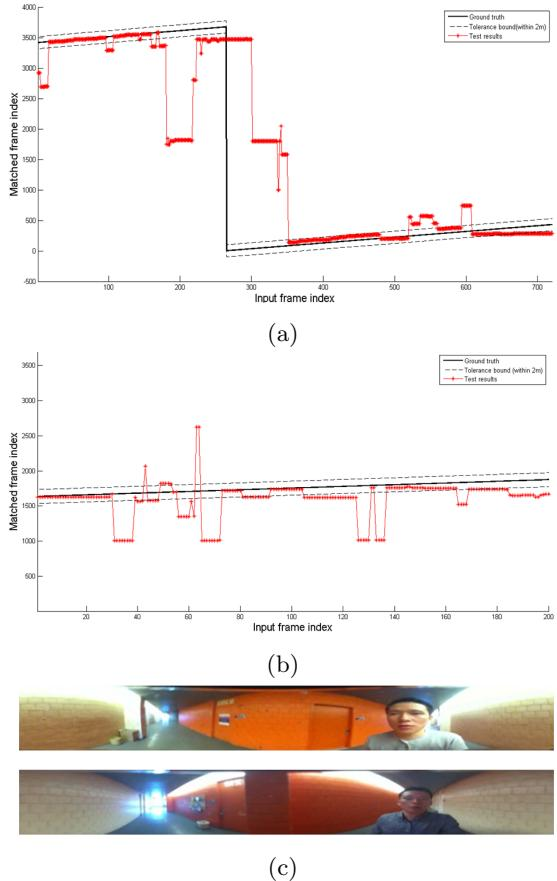
Fig. 7: (a) Matching results near the starting point of the loop; (b) matching results in the middle of the loop; (c) a pair of mismatching results
