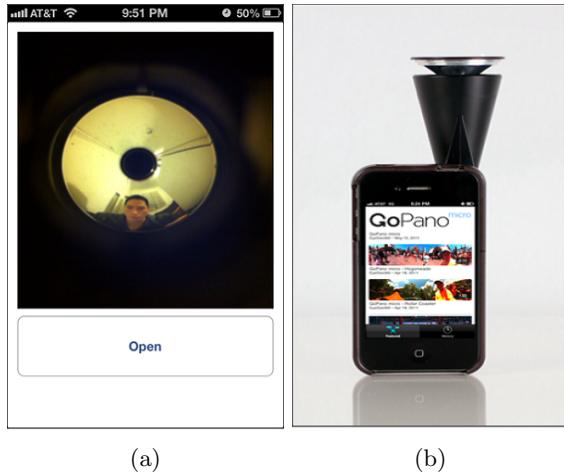
Fig. 3: Smart phone GUI and omnidirectional lens
