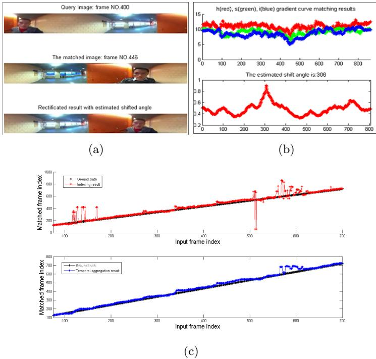
Fig. 6: (a) An example of a query image and its matched result in a database; (b) the matching scores with database frames and the estimated heading differences between the query and database frames; (c) overall matching results of all the test database frames without and with temporal aggregation
