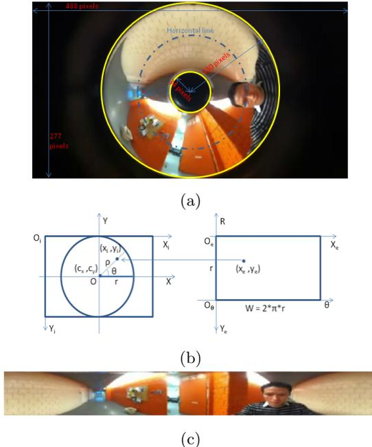
Fig. 5: (a) Original video frame and its parameters; (b) geometry relationship between the original and un-warped images; and (c) un-warped omnidirectional image
