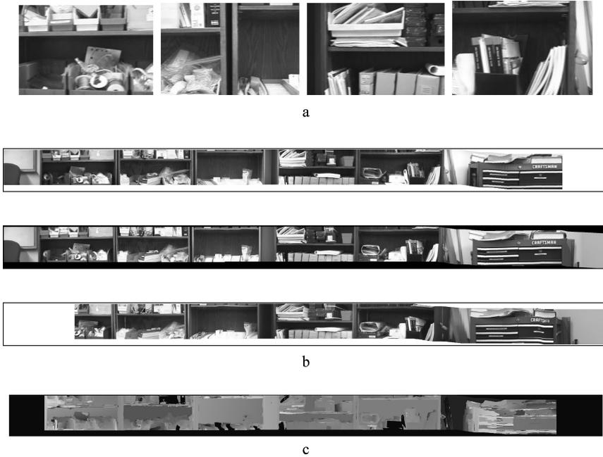
**FIGURE 12** Ground video application. (a) A few frames from a 517-frame sequence of image size  $320 \times 240$ . (b) Ground video mosaics: a left view, the center view, and a right view are shown. Each mosaic is  $4160 \times 288$ . (c) The depth map that can be used for robot navigation and target detection.
