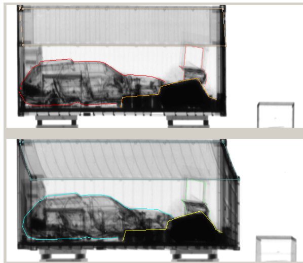
Figure 5. Interactive 3D measurements. The corresponding pairs of contours are shown in (a) and (b).
