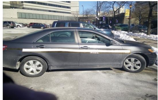
**Figure 2 long reflective tapes on the car body to record moving data.**
