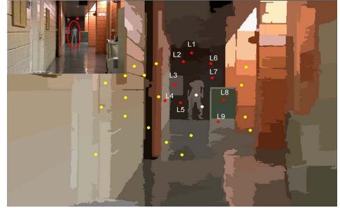
Figure 8. Interested target points close to the human target in the segmented regions are selected and labeled. Original image of the corridor (about 31 meters) under zoom factor 48 with a human target in the center (in red ellipse), is shown as an inset.
