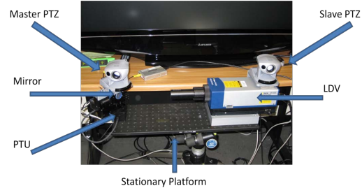
Figure 1. The multimodal sensory platform
