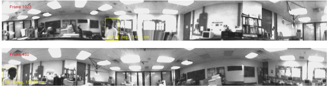
Figure 8. 3D localization by the panoramic stereo system
