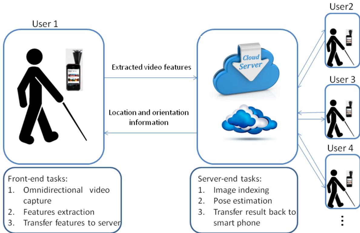
Figure 4.1: Omnidirectional-vision-based indoor localization system diagram
