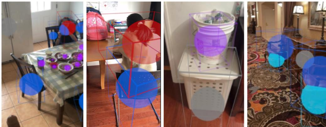
FIGURE 3.7: Examples of AR visualization of 3D object detection results. Blue represents the chair; red represents the person; purple represents the cup, bottle, and bowl; and gray represents the unknown object.
