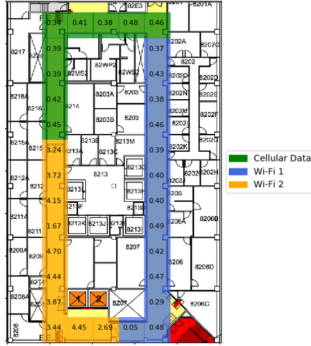
FIGURE 4.2: Download speed (Mb/s) heatmap in the corridor of the 8th floor of the NAC building at CCNY
