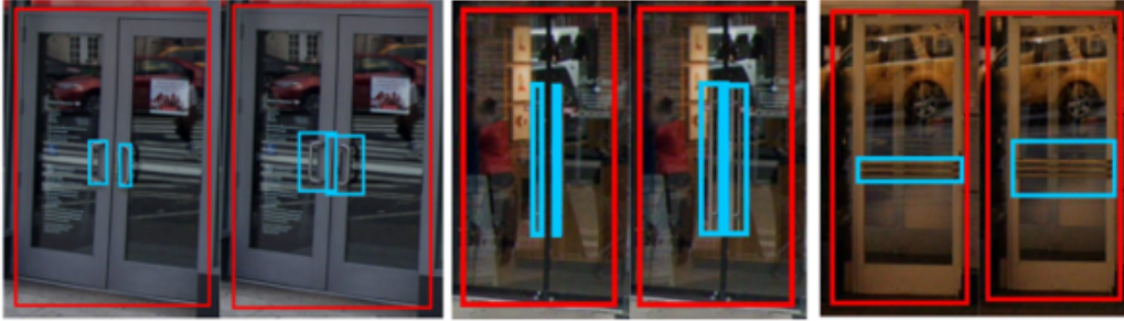
Figure 3.5: Three examples of Context in Labeling for different knob types. Left: extend both width and height. Middle: Only extend width. Right: Only extend height. In each example, the left image shows the original labels and the right image shows the extended labels.
