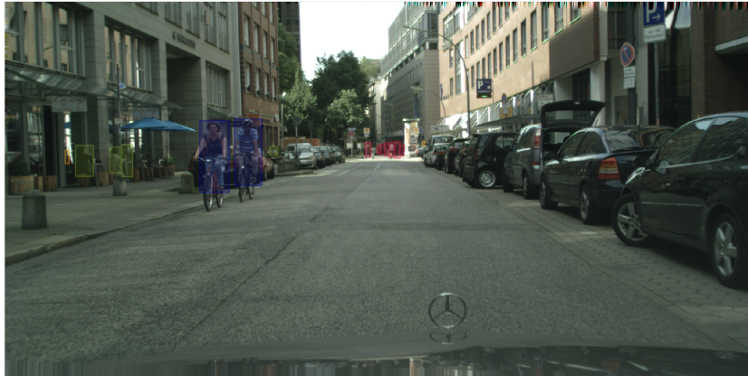
Figure 6.1: The label example from CityPersons Dataset [167]. Red: Pedestrian. Blue: Rider. Yellow: Sitting person.
