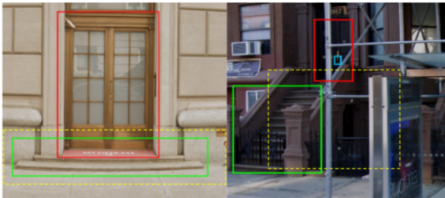
Figure 3.8: Two special cases for stair-door relations. left: door and stair have an overlapped area. Right: The stair is on the left bottom of the door due to camera perspective. Yellow dashed box: Search areas S .
