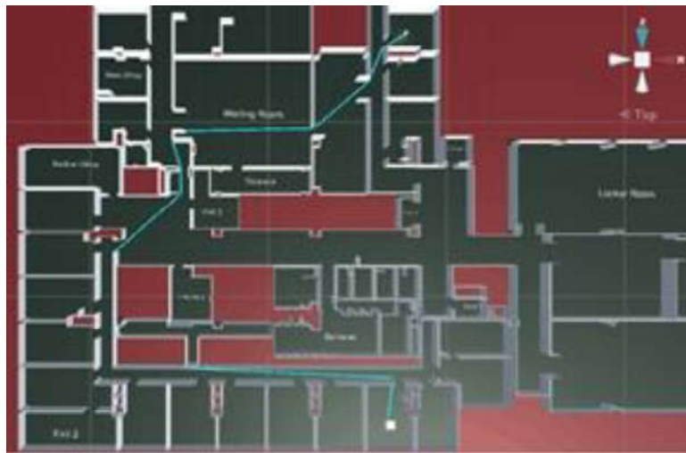
Fig. 2b. An optimal path in blue is calculated using a pathfinding algorithm. The path is connected by a few waypoints (best viewed in the electrical version).
